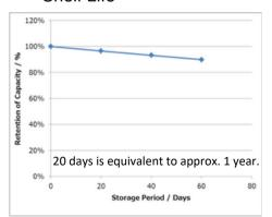
Measurement conditions:Temp:23 deg C Storage conditions: 60 deg C Dry Load: $30k\Omega$
