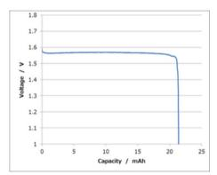
Measurement conditions: Temp: 23 deg C Load: 30kΩ
